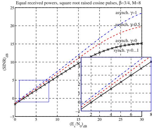
**Fig. 1:** Output SINR of a Type J-I detector with  $M = 8$  versus  $\frac{E_s}{N_0}$  for synchronous systems (lines with markers) and chip asynchronous but quasi synchronous symbol systems (lines without markers).
