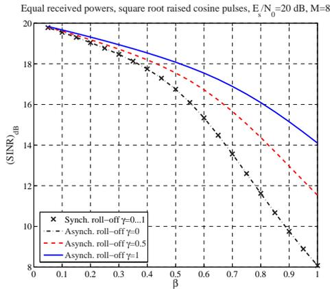
**Fig. 2:** Output SINR of a Type J-I detector with  $M = 8$  versus the system load  $\beta$  for synchronous systems (lines with markers) and chip asynchronous but quasi synchronous symbol systems (lines without markers).
