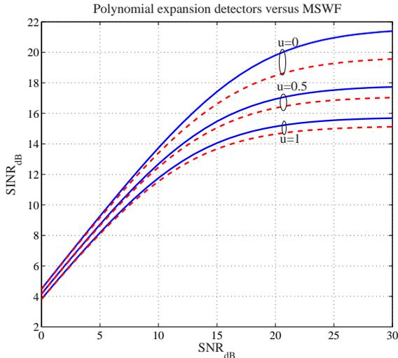
**Figure 2:** Asymptotic output SINR in decibel of polynomial expansion detectors (dashed lines) and MSWF (solid lines) with  $M = 4$  versus SNR for several coefficients  $u$  of the linear combination  $\mathbf{v} = u\mathbf{v}_{\text{MAX}} + (1 - u)\mathbf{v}_{\text{MIN}}$ .
