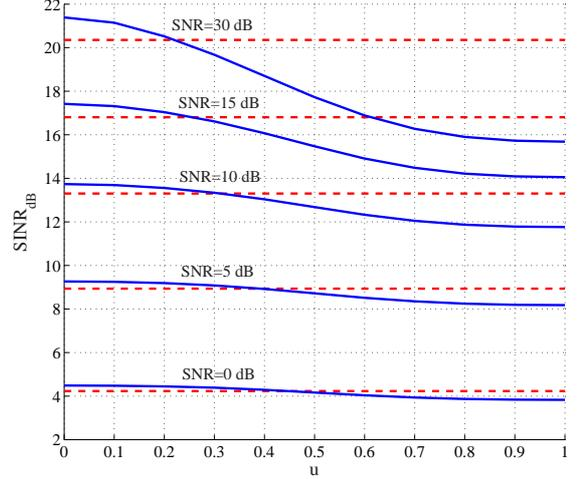
**Figure 1:** Output SINR in decibel of a Type J-I detector with  $M = 4$  versus the coefficient  $u$  of the linear combination  $\mathbf{v} = u\mathbf{v}_{\text{MAX}} + (1-u)\mathbf{v}_{\text{MIN}}$  for several values of the input SNR and correlated Rayleigh fading (solid lines) or independent and identically distributed fading (dashed lines).
